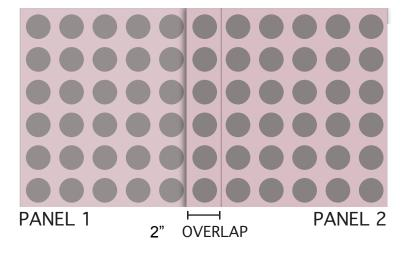
2 CUT THROUGH THE CENTER OF THE OVERLAP AREA FROM TOP TO BOTTOM USING A STRAIGHT EDGE AND A SHARP BLADE REMOVE TRIM FROM PANEL 2
